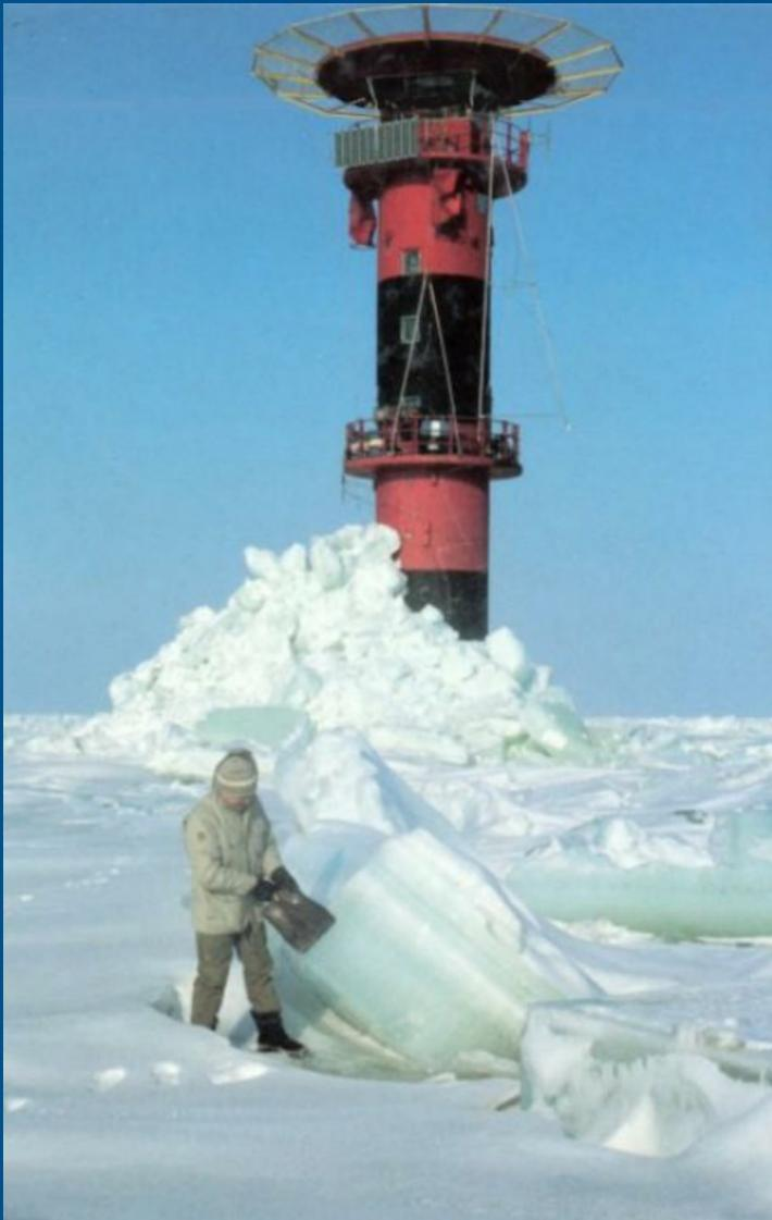
The Kemi 1 lighthouse, equipped with a force-measuring test cone, was subjected to heavy ice conditions (photo: Enqvist and Eranti, 1990).
