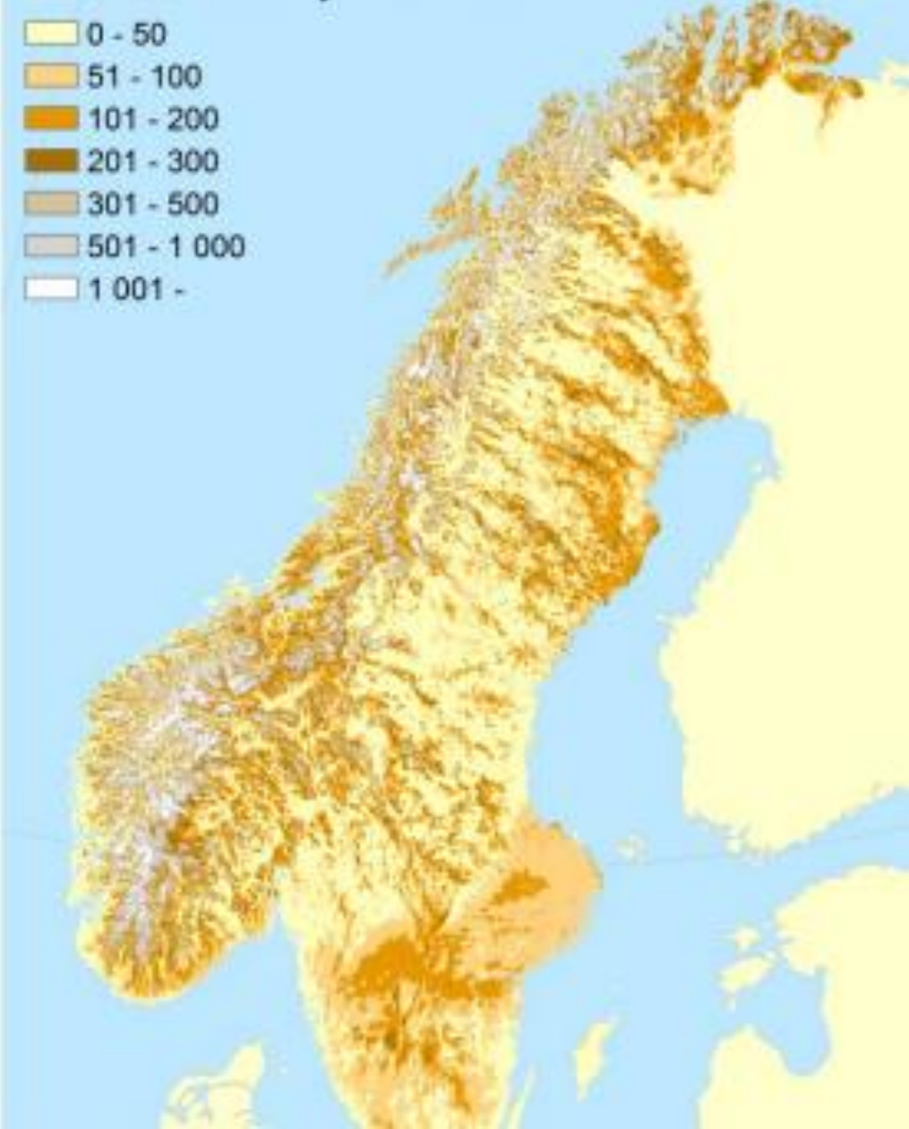
Average number of icing hours ( dM > 10g/hr ) per year given in 80 meter above ground level for Norway and 100 m for Sweden
