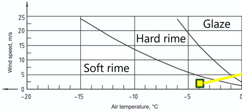
The curves shift to the left with increasing liquid water content and with decreasing object size.
