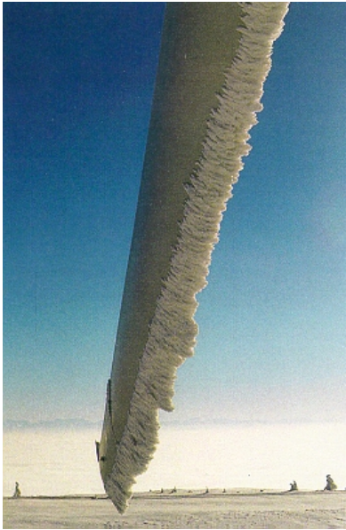
Figure 6: Heavy rime on a wind turbine blade
