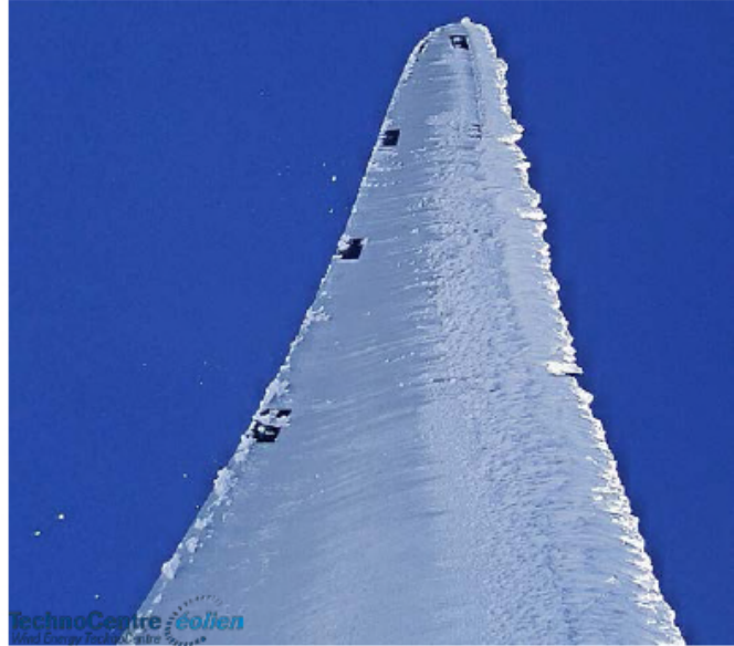
Figure 6: Heavy rime on a wind turbine blade
