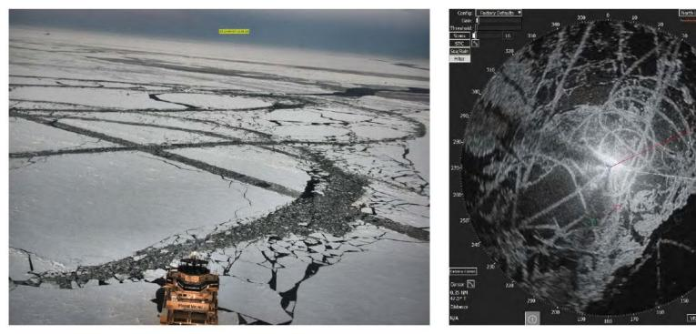
Station Keeping Trial (SKT) Full scale test; Objective to gather full-scale data on a stationary floating structure in ice.
