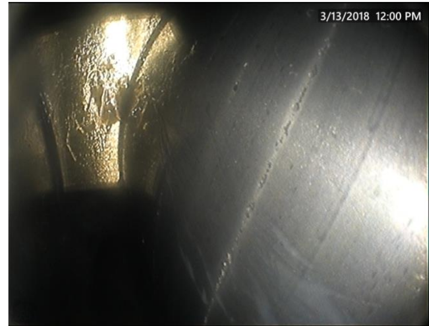
⇒ Picture: main bearing roller 5 months after REWITEC™ treatment
