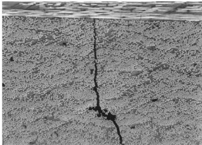
Figure 2: Optical micrograph of a [90 s /0 s ] z laminate showing microcracking after 400 thermal cycles (100X)
