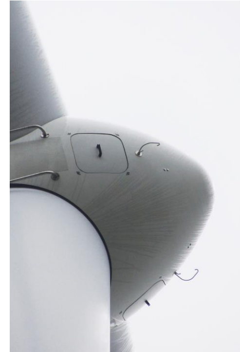
iSpin sensor mounted at the hub (Picture courtesy of ROMO Wind).
