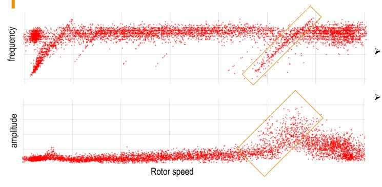
Tooth meshing frequency of the gearbox excites natural vibration Leading to resonance with high vibration amplitudes
