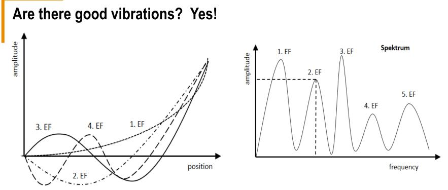
Usage of blade's vibration (EF – Eigenfrequency) for accurate ice detection
