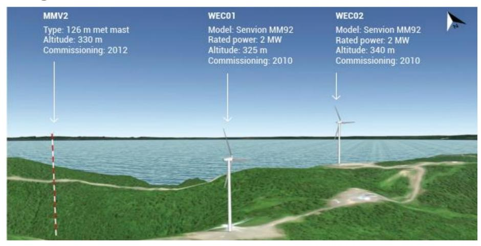
Location: Gaspe, Quebec, CA (Source: Rotor Mounted Ice Sensor – Performance Assesment by Nergica)
