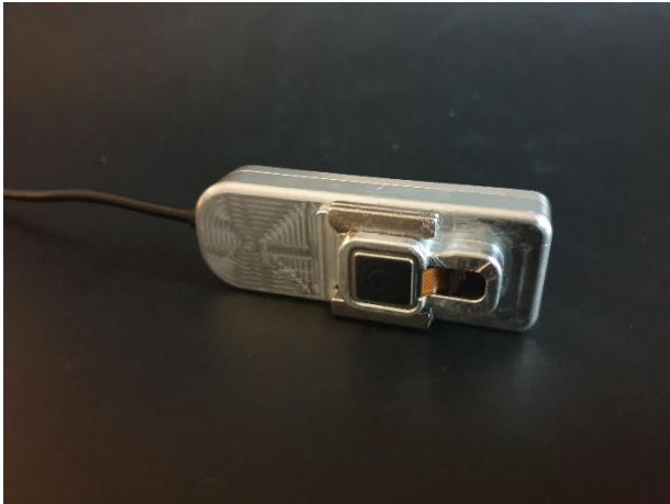
TensionCam sensor module with image sensor from Fingerprint Cards AB.
