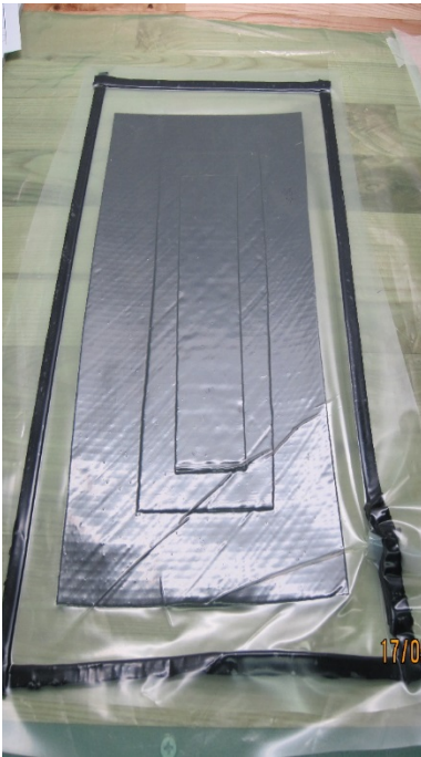
Off-blade consolidation of ply stack.
