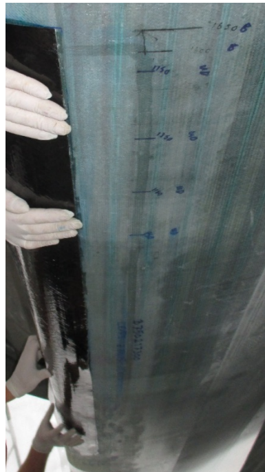
Application of ply stack to blade laminate.
