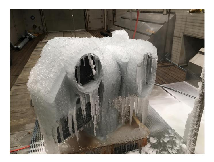
Ice test of lamp & camera module designed for offshore
