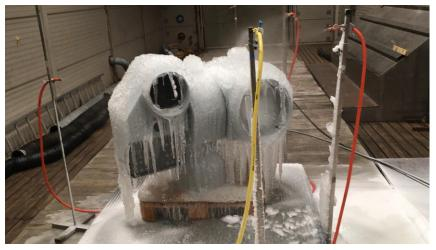
Ice test of lamp & camera module designed for offshore
