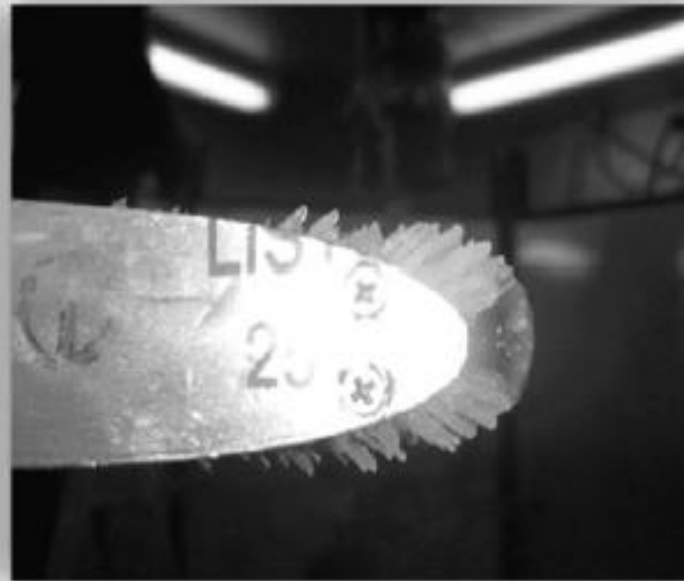
Three types of accreted ice on NACA 0012 aerofoil (Han et al., 2012)
