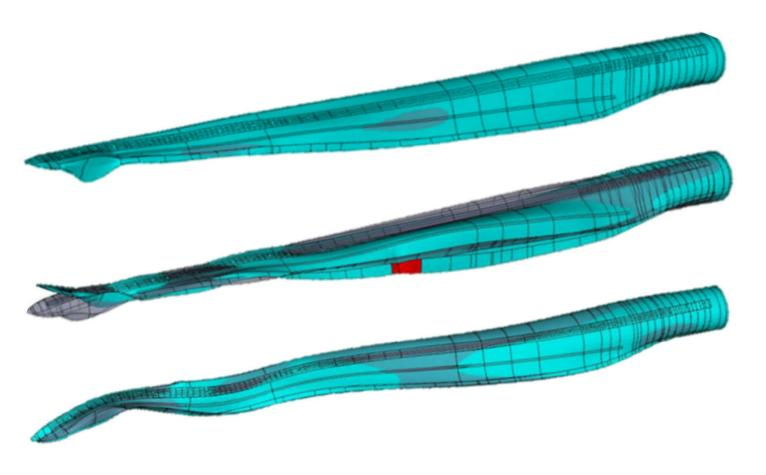
Rotor blade vibrations give us information about the state of the structure:
