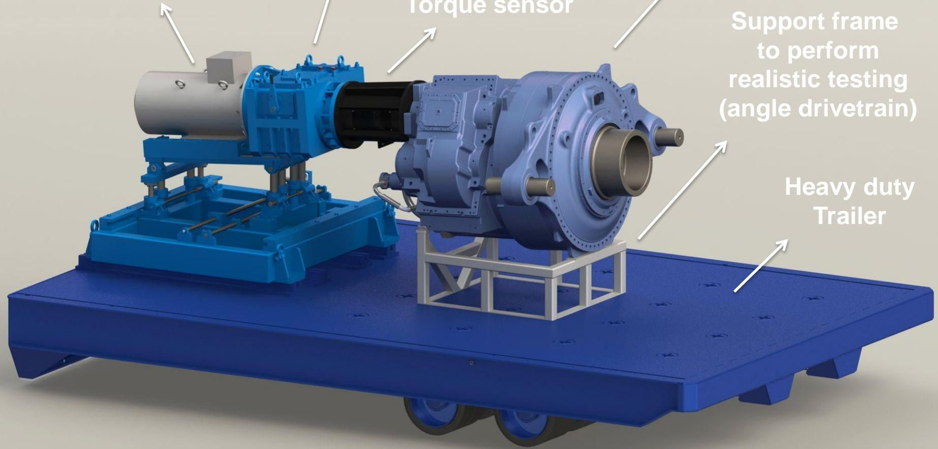
**Cold start-up test bench – 10 kNm torque**
