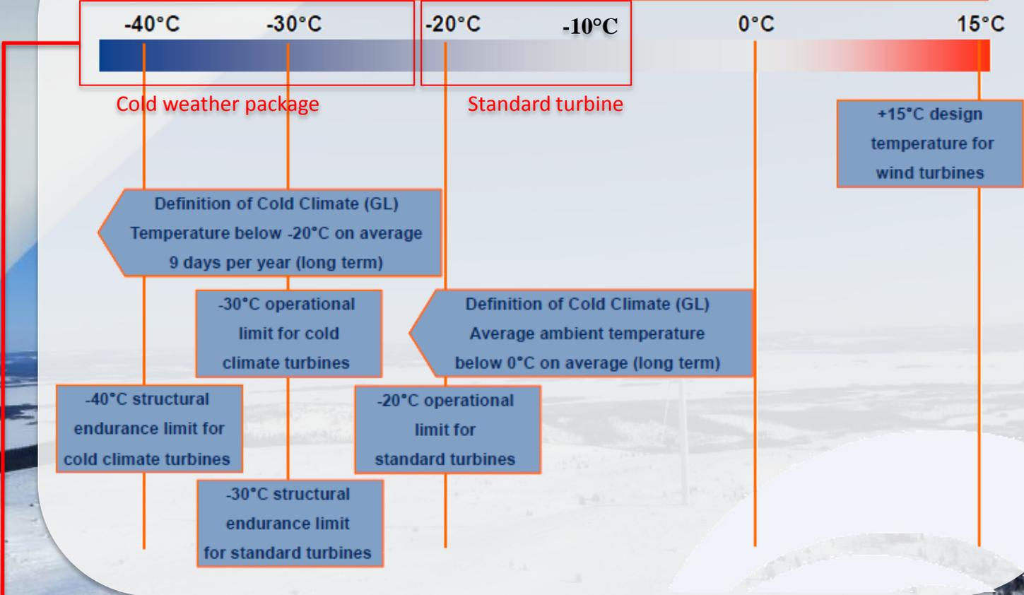
“Extend temperature ranges, using 200 kW to 300 kW parasitic power per turbine at conditions below -20C for heating components such as the nacelle space, yaw drive and pitch motors, and the gearbox, slip ring, controller and control cabinet, and battery”
