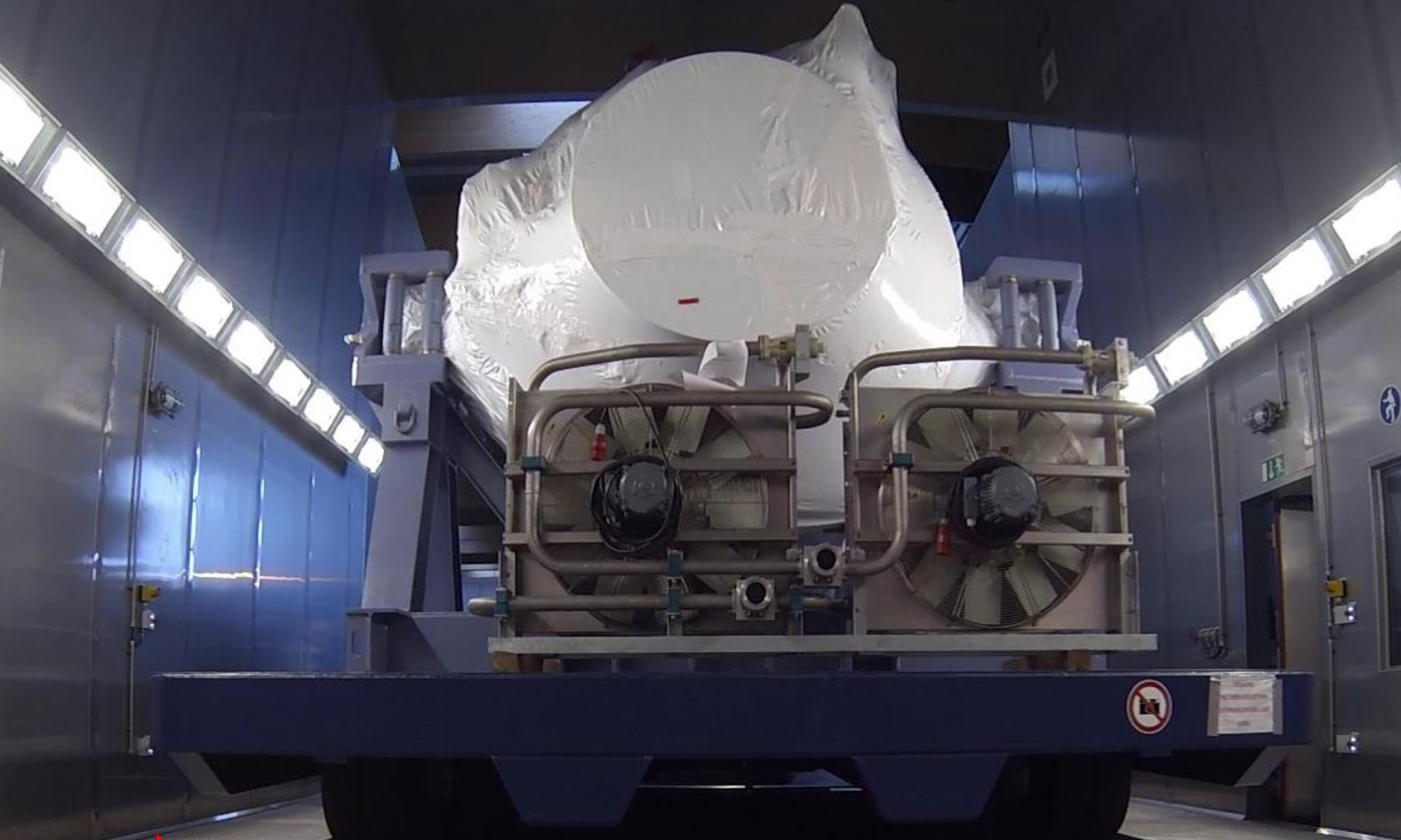
**State-of-the-art CCV gearboxes are tested for worst case scenario's: failing heater ; grid fall ; cold-start**
