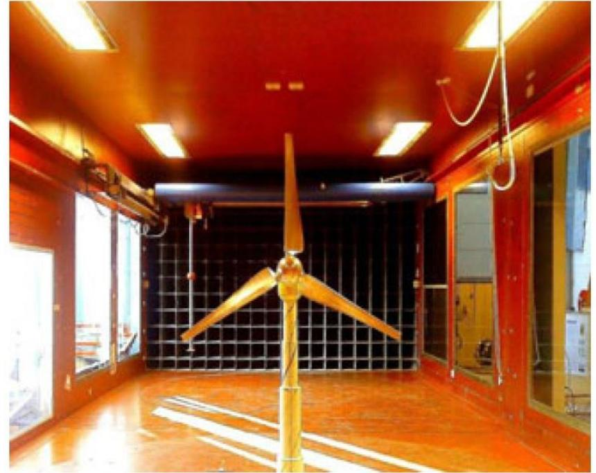
Model mounted in the wind tunnel
