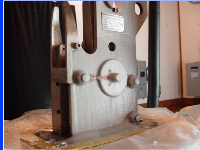
Lifeboat Hook with Icing Accumulation
