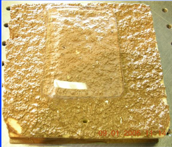
Clear Ice Layer on Space Shuttle Foam
