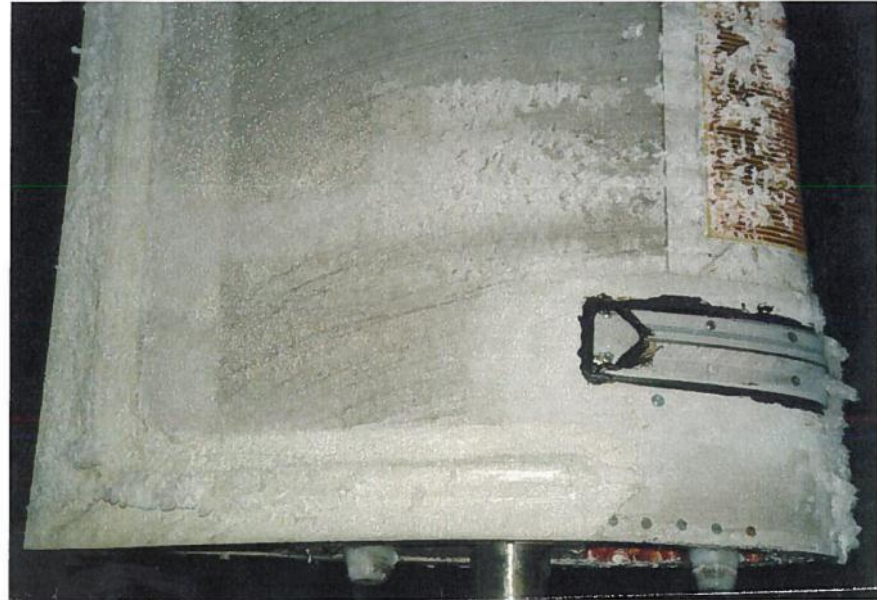
Figure BF. The first blade mounted ice detector delivered by Labko Oy. Pyhätunturi test station 1994.
