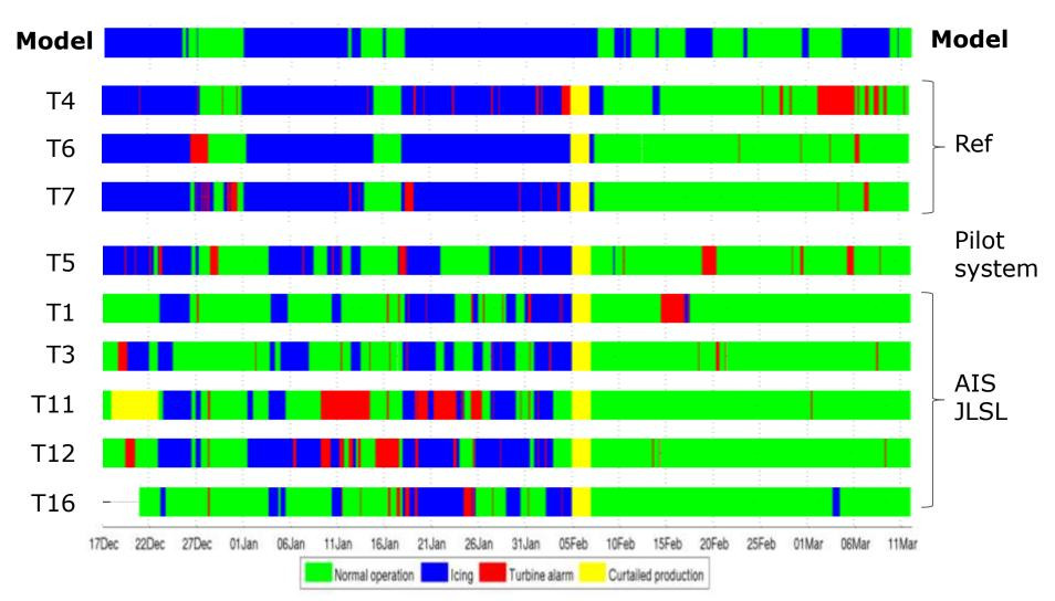
Significantly less icing induced power losses on AIS turbines
