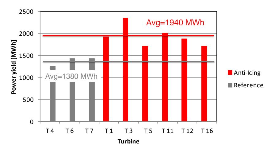
On average **560 MWh higher production with Anti-Icing Option** compared to reference turbines from CW51-CW10
