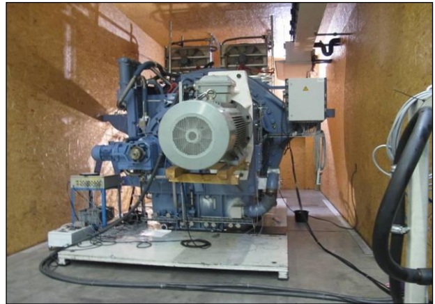
Figure 6: Cold start test ZF Wind Power Gearbox
