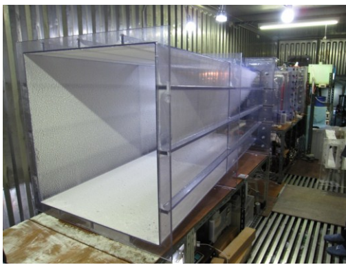
Figure 3. Icing wind tunnel set-up provides cloud droplets with airflow under sub-zero temperatures.
