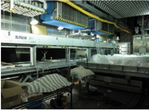
Figure 1. Snowing wind tunnel set-up. Fresh snow is fed to snowfall device from where it falls down to the wind tunnel, where the unit under test is located.
