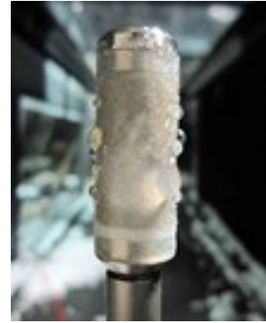
Figure 2. Ice bridge forms to original transducer design in the snowing wind tunnel.
