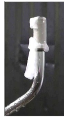
Figure 4. Ice growths from unheated structures of the original transducer design in the icing wind tunnel.
