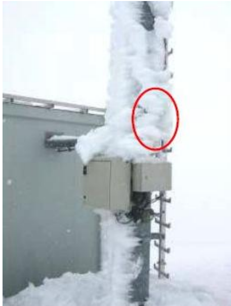
Temp.-/humidity sensor at a test rig (red circle), © Lachinger, 2011
