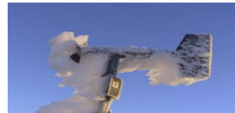
Heavily iced anemometer, © Cattin, 2008
