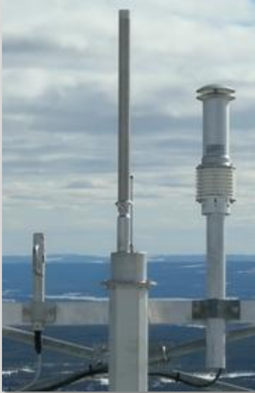
Ice detector, ice load, met sensor
