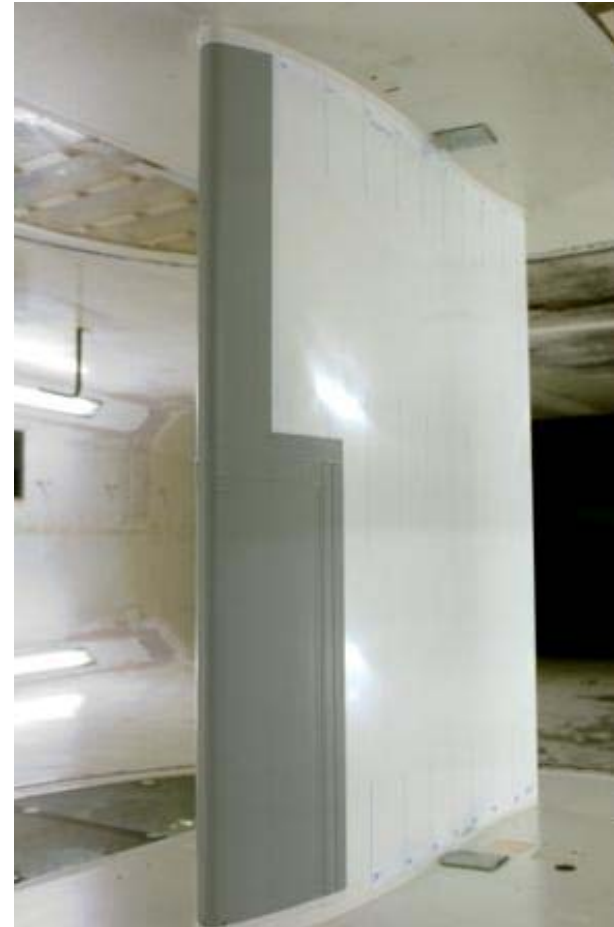
Active de-Icing system – wind tunnel test
