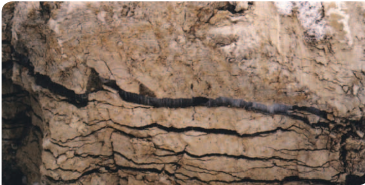
Figure 5. Ice lens in a silty soil.
