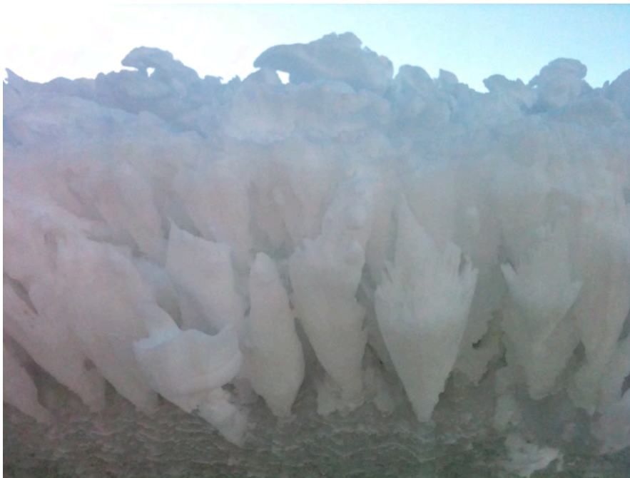
Figure 1: Ice build-up along the leading edge of the blade. This turbine has since long stopped producing.
