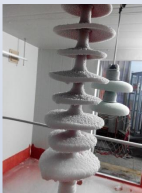
(c) Insulator icing graph
