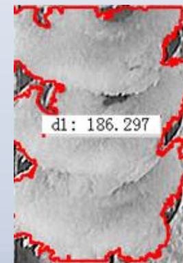
(f) Iced Insulator diameter
