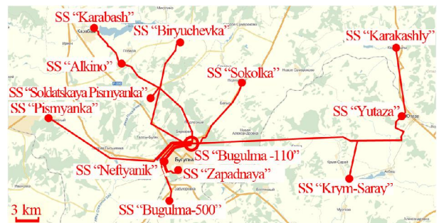
Figure 4. A schematic arrangement of seven power transmission lines of substation "Bugulma-110" controlled by radar complex
