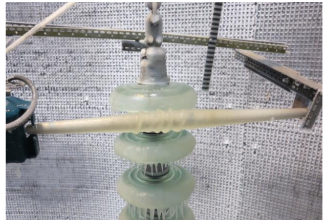
Figure 6: Example of ice accretion at the rotating rod, when the rod was installed on top of the insulators.
