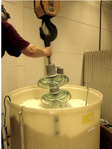
Figure 3: Example of application of pollution by dipping of the insulators (IEC 61245).
