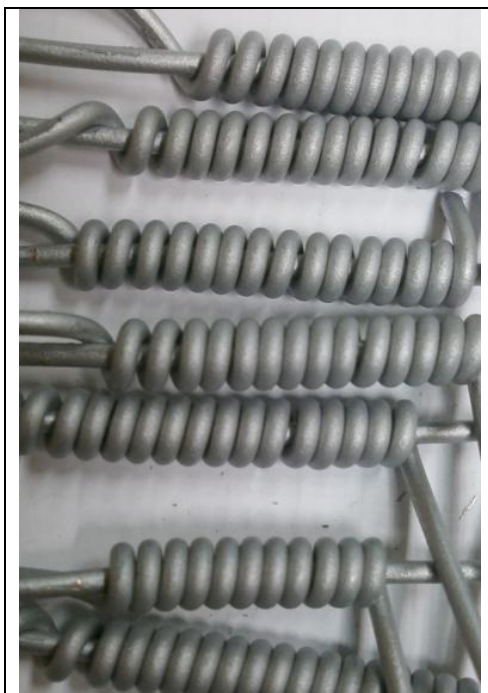
Fig 07 : Quality test of coating: the "tie" test
