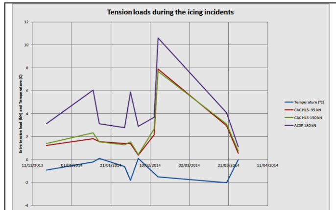
Fig 12 : Overview of stress increases experienced by strand coated CAC and uncoated ACSR..
