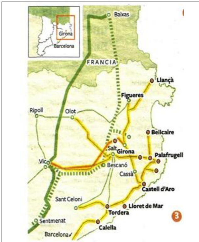
Fig 03 Detail of the most affected area, highlighted in yellow the affected set of distribution lines
