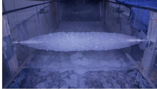
Figure 1 Accumulated atmospheric ice on the rotating cylinder
