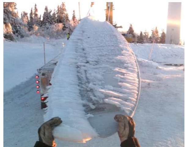
Figure 1: Ice collected on a wind turbine blade, which was taken down for the removal of a de-icing system.
