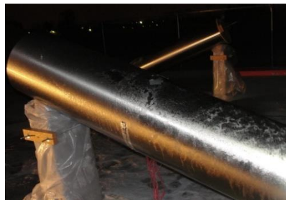
Figure 9: Formation of Ice in Chemical Anti-icing Test
