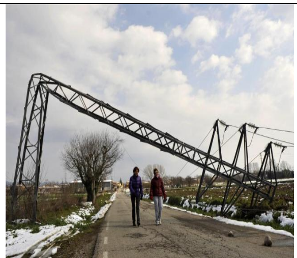
Fig 05 : Tower of 25kV line , 2 circuit, collapsed by the weight of the snow
