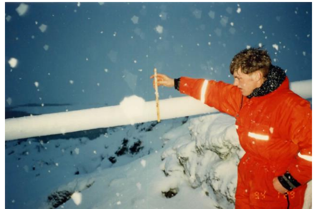
Figure 6: Observing and measuring a diameter of wet snow accretion in southeast-Iceland.
