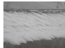
Fig. 7 Relationship between ice shape of 3-bund conductor and time
