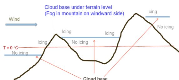
Figure 2. Schematic influence on cloud base and rime icing from upwind mountain topography.
