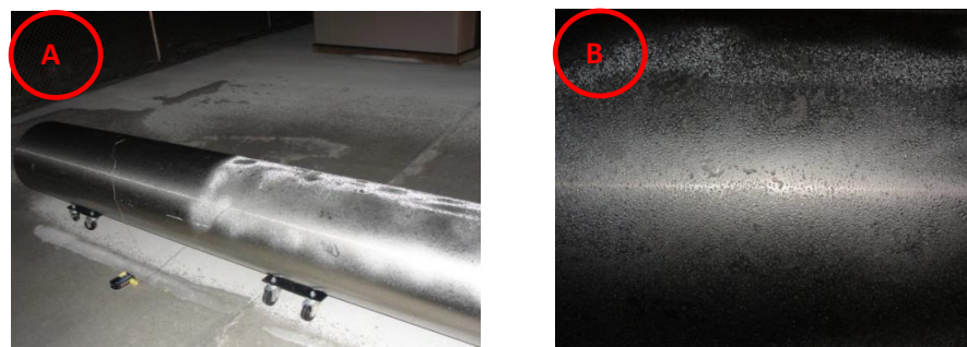
Figure 5: A) Aliphatic petroleum distillates with Proprietary additives Sprayed on half of the Specimen, B) Water Droplets due to aliphatic petroleum distillates with Proprietary additives
