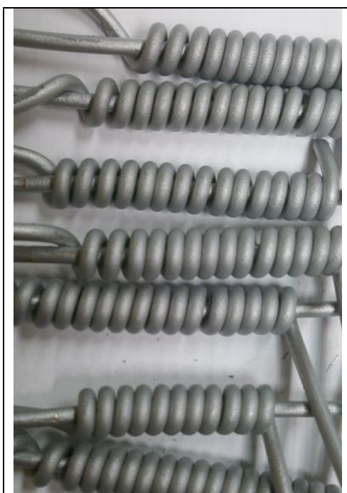
Fig 07 : Quality test of coating: the "tie" test
