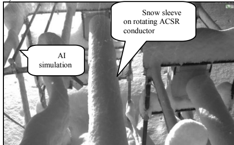
Figure 16: wet-snow accretion on the rotating conductors (photo taken 1-hour before snow shedding, 05-02-2015 06 UTC). In the upper left of image, the two AI conductors are free of snow sleeve.
