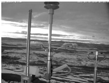
Figure 3: A view of the instruments at the Sjisjka icing measurement station. This particular mast is 60 m tall.
