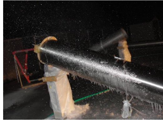
Figure 7: Accumulated Ice in Anti-icing Thermal Test
