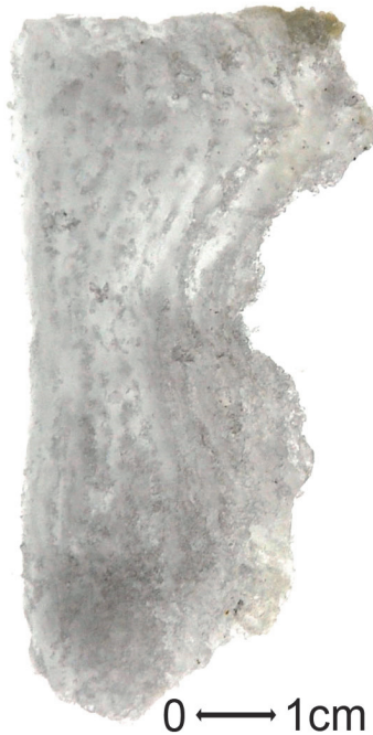
Figure 5: cross section of a sea spray ice sample.
