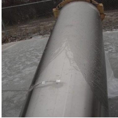
Figure 6: De-icing Pattern in Thermal Test
