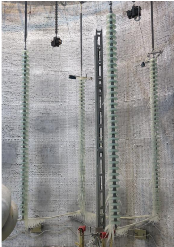
Figure 9: View of the insulator strings covered by glazed ice accreted under full DC voltage 361 kV.
