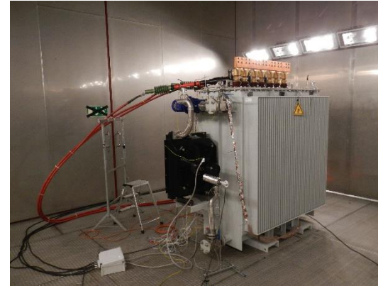
Full functional electrical tests with or without wind turbine auxiliaries (forced cooling, pumps, heating, expansion tank,...)
