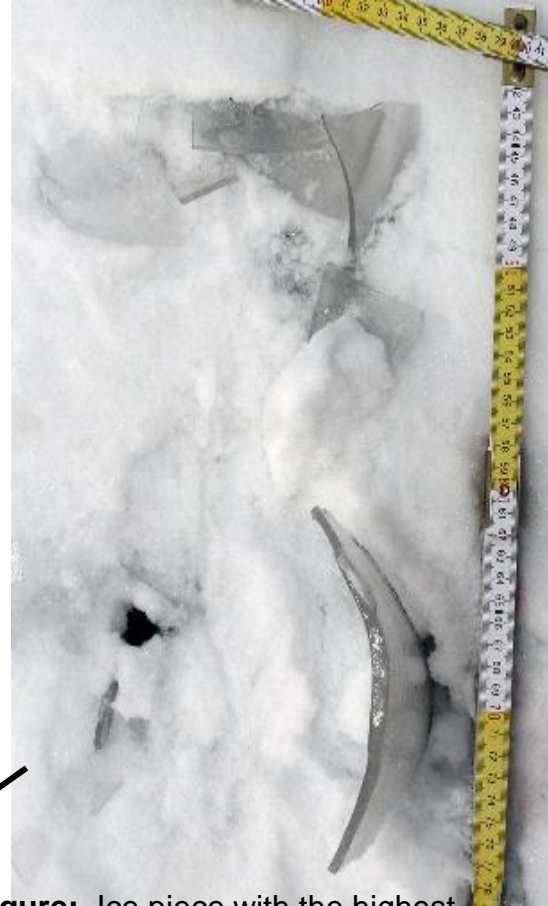
Figure: Ice piece with the highest recorded shed distance of 225 m from a turbine with 138 m hub height and 82 m rotor radius. The length of this piece was 38 cm, the width 16 cm and the thickness varies between 3 and 8 mm. It was pure glaze ice with a weight of 240 g.
