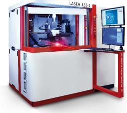
Laser textured surfacing, is an innovative manufacturing technique based on laser technology for creating simple or complex patterns on existing surfaces
