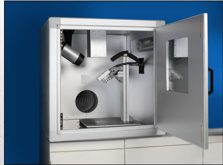
(2) Ice rain test: Simulates water run-off and subsequent formation of clear ice
