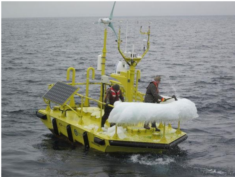
Example: ice removal on floating lidar buoy
