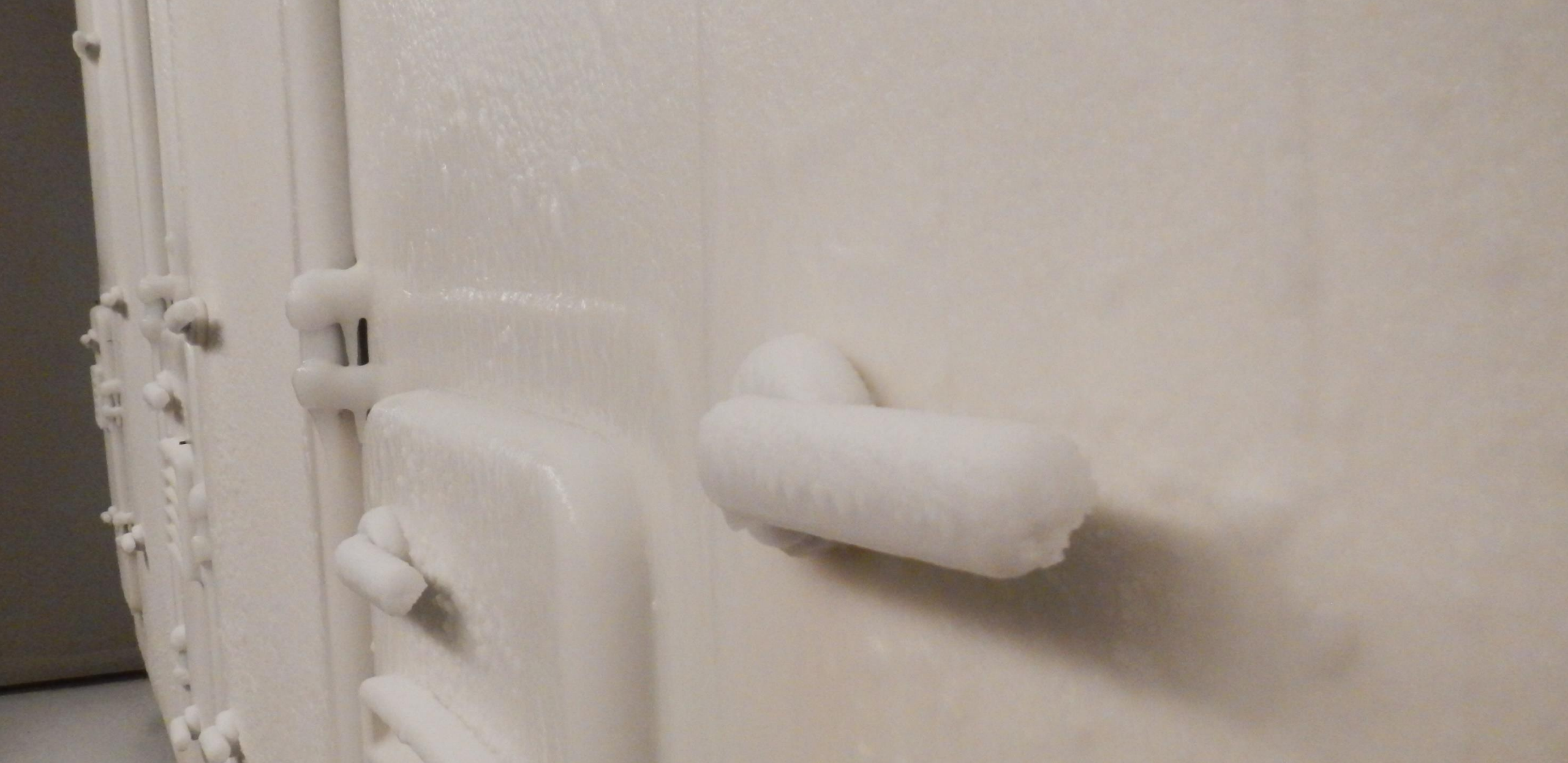
Icing tests in the climate chamber
