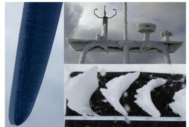
Ice Class Rime 5 (ICR5) – 2.8 to 5.0 kg/m
