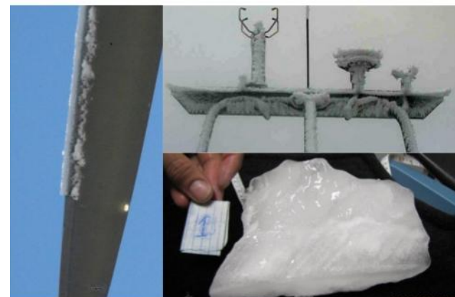
Ice Class Rime 5 (ICR5) – 2.8 to 5.0 kg/m
