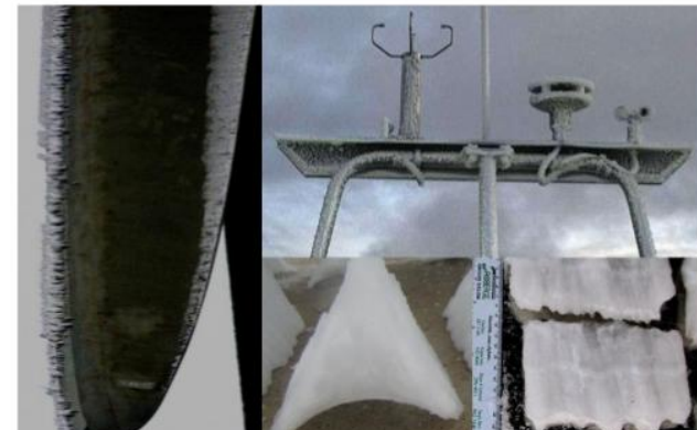
Ice Class Rime 4 (ICR4) – 1.6 to 2.8 kg/m
