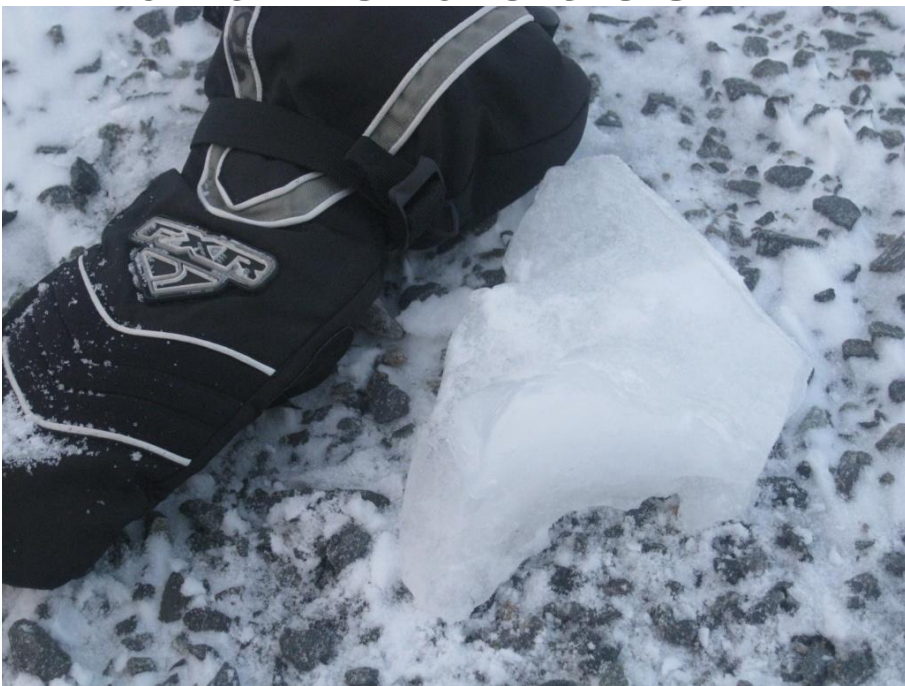
Icepiece found 25 m from tower of turbine. Kjøllefjord, Norway 29.march 2008.
