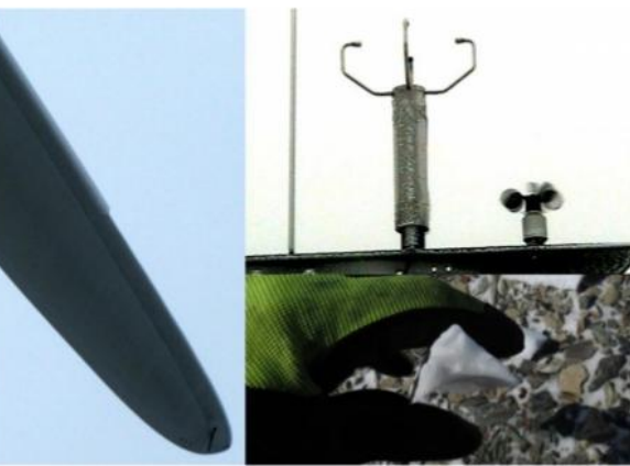
Ice Class Rime 1 (ICR1) – 0 to 0.5 kg/m
