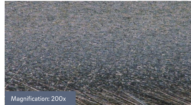
Microscopy bearing ring, Castrol X320 without REWITEC®
