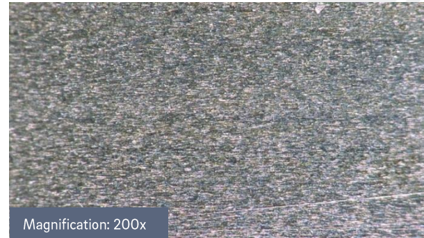
Microscopy bearing rolling elements, Castrol X320 with REWITEC®
