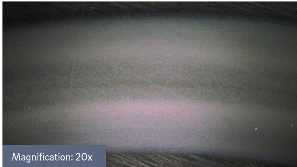
Microscopy bearing ring, Castrol X320 with REWITEC®
