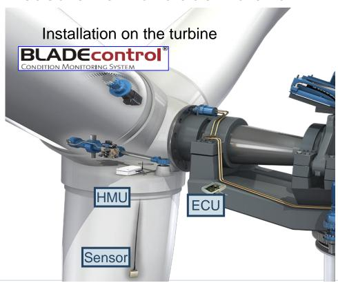
Precise detection of icing for automated turbine shutdown and restart
