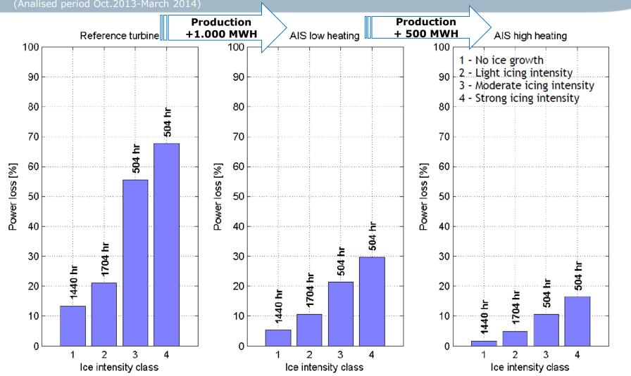
Production loss in 4 ice intensity classes for reference turbine (left), AIS with low heating (middle), and AIS with high heating (right). The number of hours with icing in the different classes is also shown.
