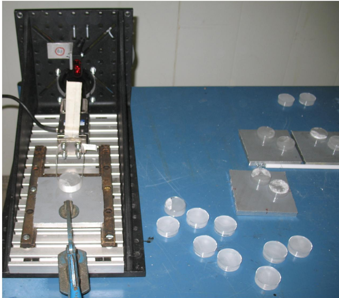
VTT basic ice adhesion tester /4/
