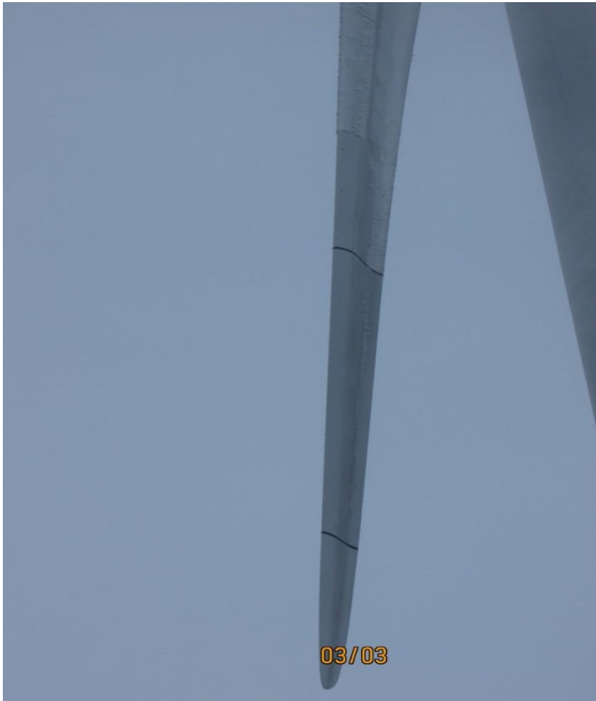
Blade after de-icing cycle
