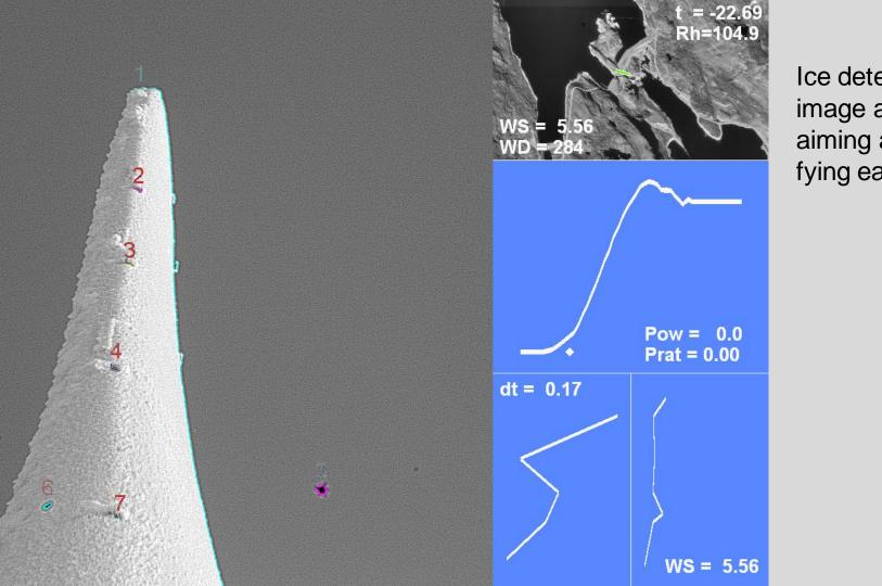
Ice detected by image analysis, aiming at identifying each reflex.
