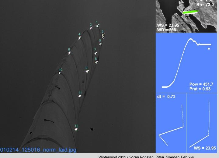
Ice detected by image analysis, aiming at identifying each reflex. More reflexes... under operation. Easier at night. Long exposure.
