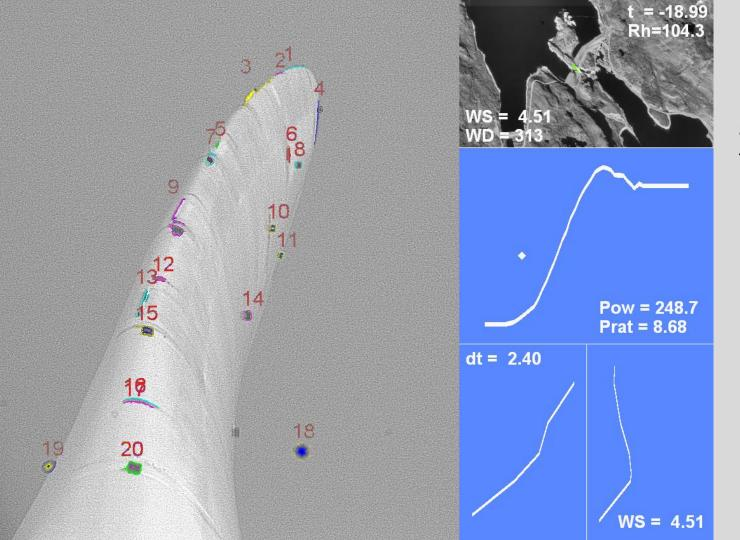
Ice detected by image analysis, aiming at identifying each reflex. More reflexes... under operation.
