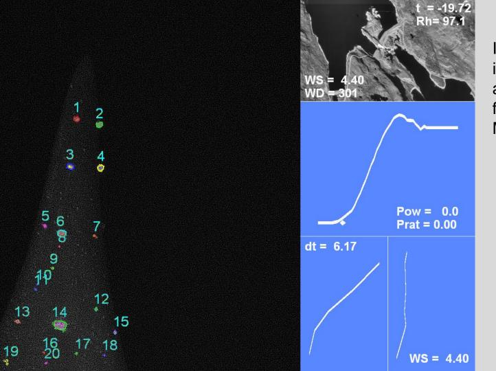
Ice detected by image analysis, aiming at identifying each reflex. More reflexes...
