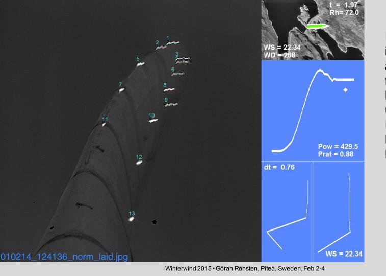
Ice detected by image analysis, aiming at identifying each reflex. More reflexes... under operation. Easier at night. Long exposure. Longer exposure.
