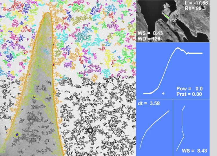
Ice detected by image analysis, aiming at identifying each reflex. More reflexes... under operation. Easier at night. Long exposure. Longer exposure. Colours?
