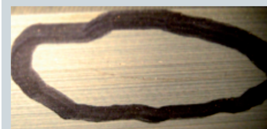
Example: Hairline fracture in tooth. If the tooth section breaks off it could damage other components, causing turbine stop and costly repairs.
