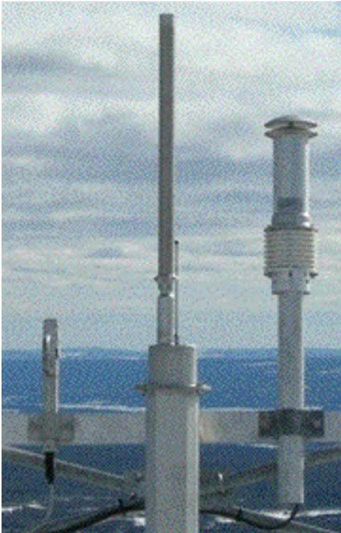
Ice detector, ice load, met sensor
