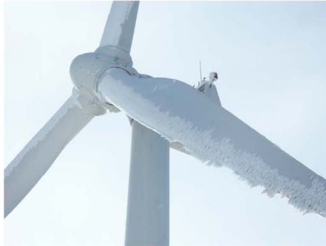
Icing on an NM82 (V82) in Aapua, Övertorneå municipality in the county of Norrbotten, Sweden, From Mapping of icing for wind turbine applications by Göran Ronstein, Elforsk 2008
