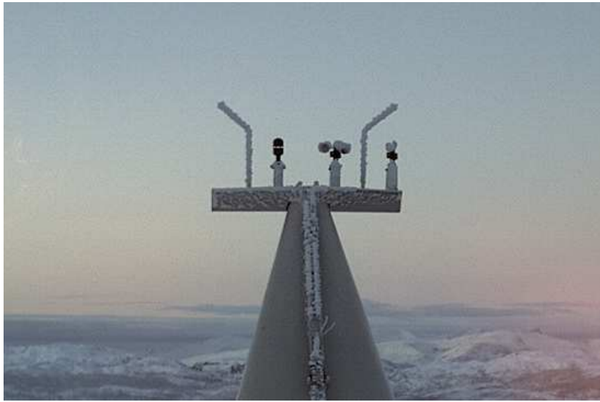
Fig. 6. Rime ice visible on the sensors following the icing event Dec. 5.
