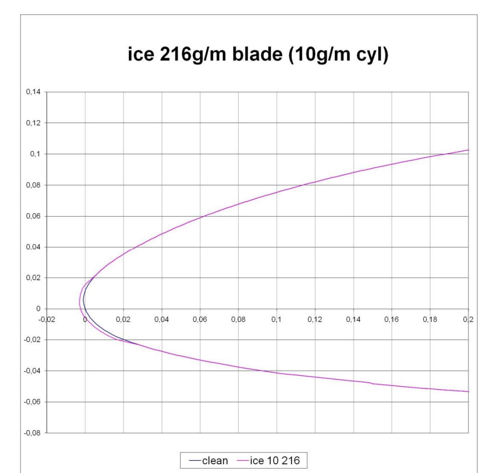
Figure 1: Iced and clean profile and ice mass (~200g/m), in the conditions similar than producing 10g/m ice on standard cylinder.
